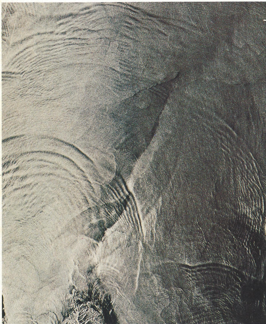
In the Gulf of California, Baja Mexico, a SEASAT synthetic aperture radar image shows the northern tip of an island at bottom left. The pronounced concentric bands are internal waves,
